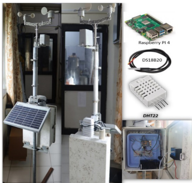
Mini weather station fabricated with Wireless weather sensors (DHT22, DS18B20 and weather meter kit)
